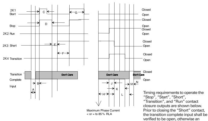
Steps A to F: Starter Integrity Test.
